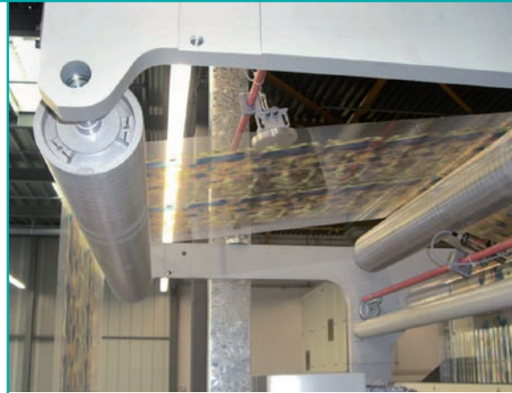
Static Multi Monitoring ahead of winding a film web
