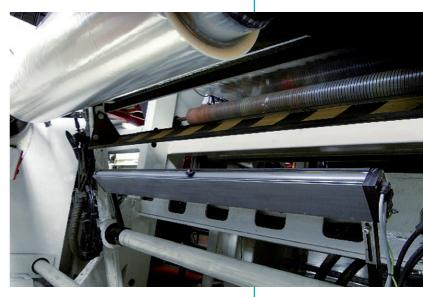
Non-wearing emission tips, robust and an easy-to-clean design ensure that only a minimum of maintenance is needed. An aluminum profile on the rear with cage nuts makes for easy assembly, even in difficult installation situations.
